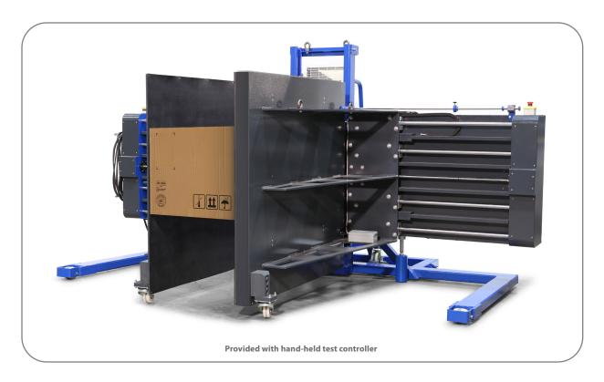
Severe horizontal compressive forces occur when packaged products are mechanically handled at different points within the supply chain. Packages can also experience damage-inducing horizontal compressive forces in both the e-commerce and parcel environments as fast moving packaged products accumulate at various points in those supply chains.
