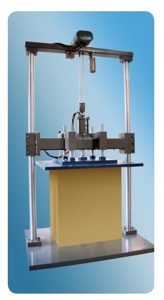
Severe compressive forces occur when packaged-products are stacked during transit or storage. To evaluate the performance of packages, components, and materials under such loads, Lansmont offers a full line of Compression Testers. Lansmont Compression Testers comply with industry standard package testing specifications including ASTM, ISTA, ISO, and MIL-STD.
