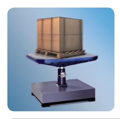
The Model 1800 Vibration Test System will perform a wide range of testing applications. The system runs resonance search and fixed-frequency dwell tests for product evaluation. Additionally, the 1800 is used for distribution simulation, referencing ASTM, ISTA, ISO and other common industry test specifications, as well as test profiles created from SAVER™ environmental data.
