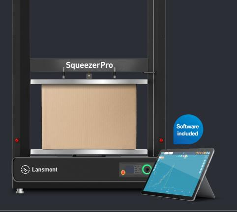
Crafted to evaluate box performance, SqueezerPro offers powerful insights into the compressive strength performance of various board mediums, closures, interior partitions, and other critical design variables. Additionally, SqueezerPro can be used to conduct distribution simulation compression testing for individual packages.
