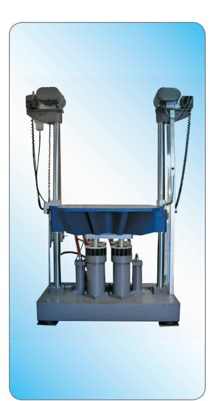
The Model 122 Shock Test System payload capacity and large table size make it a versatile platform for testing larger products or for testing multiple items simultaneously. The Model 122 is available in standard and heavy-duty configurations to tailor the system to specific applications.
