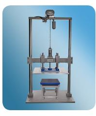
Testing Individual Packages For testing smaller items such as individual packages, an optional package test stand can be used with the Model 122-15. A Low Range Load Platform is another useful option for accurately evaluating low level force inputs.
