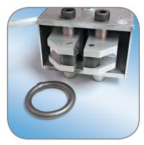
The QR 3000 consists of a quick-release mechanism, lifting ring, and foot switch for initiating the drop. Straps wrapped around the test item form a sling that is attached to the lifting ring, which is placed in the jaws of the quick-release mechanism. The quick-release mechanism and package are then lifted
