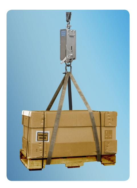
Lansmont's QR 3000 drop tester simulates the drops and impacts that occur in distribution. It is especially suited to very large, heavy payloads which cannot be tested on conventional drop test machines. The QR 3000 can perform free-fall drops (flat, edge, and corner) on packages of virtually any size and shape.
