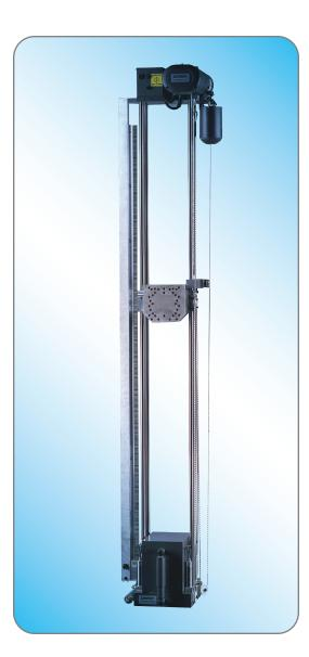
The Model 23D Shock Test System is a high-performance version of the Model 23 Shock Test System. The multi-sided magnesium shock carriage generates nearly ideal half-sine shock pulses and allows for mounting test items in multiple orientations simultaneously.
