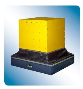
Giving you the ability to replicate vibration environments with full 6 degrees of control, Lansmont has taken vibration testing to a whole new level. An advanced technology vibration test system that offers 6 Degrees of Control, the CUBE™ can accurately replicate many vibration environments with precise digital control.
