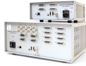
provides capabilities to define test constraints for electrical connections and determine when those design constraints have been exceeded.
